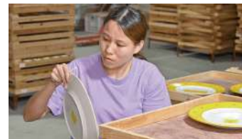
Applique-Semi-finished Product Quality Inspection
